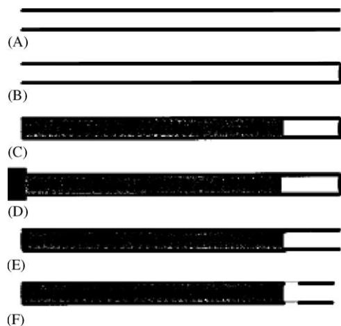
Fig. 15. Preparation of a sol–gel mediated monolithic CEC capillary: (A) 60 cm of hydrothermally pretreated 50 μm i.d. fused silica capillary; (B) closure of the distal capillary end via an oxyacetylene torch; (C) filling 50 cm of the capillary with the sol–gel solution using 100 psi helium pressurization; (D) closure of the proximal capillary end via a 60 s epoxy glue, followed by thermal conditioning; (E) opening of both capillary ends via an alumina wafer following the completion of thermal conditioning; (F) preparation of an UV detection window just adjacent to the termination of the monolithic matrix. Adapted from [100].
